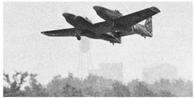
The North American F-82G. An unlikely marriage of a pair of Mustang's on a common wing. Art Johnson's R/C Scale. It flew well. 91" span, 18 lbs. Kraft receiver, Heathkit transmitter, Rhom Air retracts, Hydra-Lock. Postwar era.
