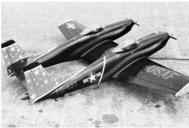
The North American F-82G. An unlikely marriage of a pair of Mustang's on a common wing. Art Johnson's R/C Scale. It flew well. 91" span, 18 lbs. Kraft receiver, Heathkit transmitter, Rhom Air retracts, Hydra-Lock. Postwar era.
