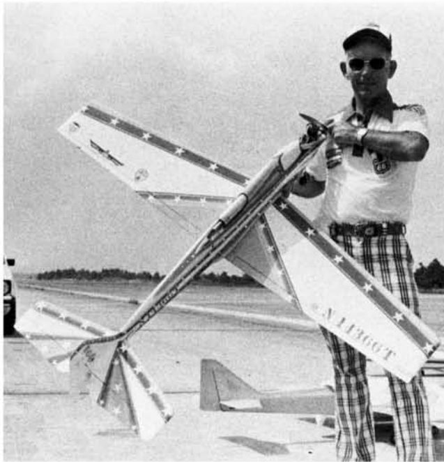
3 Perfection. Bill Thomas' aircraft. Fox Hawk. OPS pipe, Goldberg retracts. Sonic actuators, EK Logictrol radio. Tuned pipe faired within the fuselage. Center right: Joe Whelan cranks his machine to life. Tense moment for flyer. Right: A modified Compensator by Ed Hartley of Knoxville. Rhom Air retracts.
