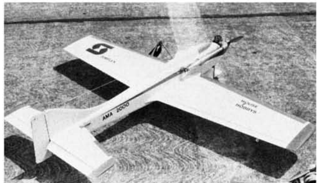
3 Perfection. Bill Thomas' aircraft. Fox Hawk. OPS pipe, Goldberg retracts. Sonic actuators, EK Logictrol radio. Tuned pipe faired within the fuselage. Center right: Joe Whelan cranks his machine to life. Tense moment for flyer. Right: A modified Compensator by Ed Hartley of Knoxville. Rhom Air retracts.
